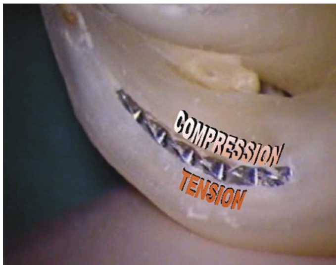
Fig. 18.16. Bending stress: on the internal aspect of an instrument rotating in a curved canal compression develops while on the external aspect tension develops. In the centre of the instrument there is theoretically a neutral zone that does not develop stresses.
