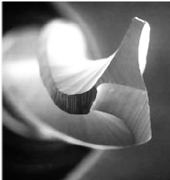
Fig. 26.43. Scanning Electron Micrograph of the tip of a pro Post Bur (Dentsply-Tulsa Dental); the oblique cut of the tip is very aggressive and is able to cut and remove the carrier with precision.
