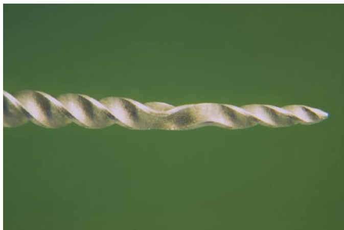
Fig. 18.34. ProFile .06 with visible plastic deformation.
