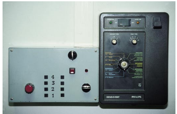
Fig. 5.95. This Philips timer (right) is used to automatically regulate the exposure time according to the teeth being treated. A switch (left) allows a single timer to control several X-ray machines in different rooms.
