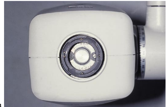
Fig. 5.9. A. The aluminum filter interposed in the X-ray path impedes the soft rays with long wavelength and low penetrating power, which are useless and damaging (continued). B. Disassembling the long tube, the aluminum filter is visible in the exit portal of the X-rays.
