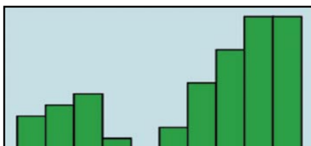
Digital transformation of luminosity The sampled value is calculated on the mean point of intervals.
