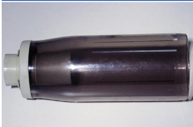
Fig. 5.10. A. The collimator reduces the diameter of the X-ray beam, thus diminishing the volume of the tissues irradiated and thus the production of secondary, useless, and damaging radiation. B. The metallic tube visible within the long tube collimates the X-ray beam.
