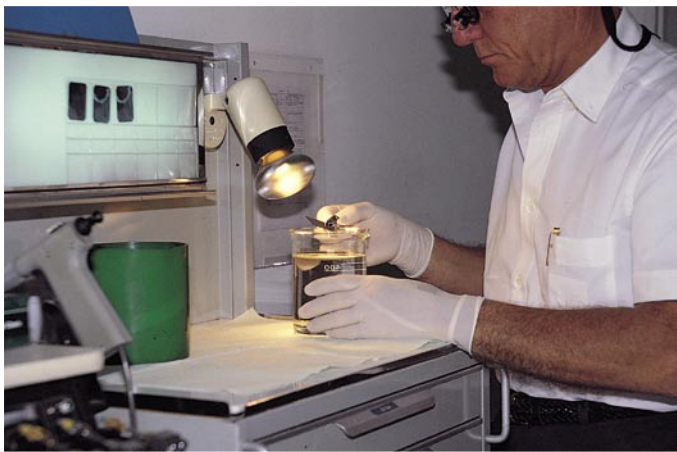
Fig. 5.88. Although barely immersed in the fixer and removed from the dark room, the radiograph can be read by incident light. It is illuminated from above by the lamp of the unit or a light on the cabinet.
